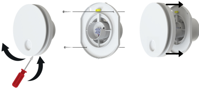
FIG.1 - Remove the grille from the motor housing.
