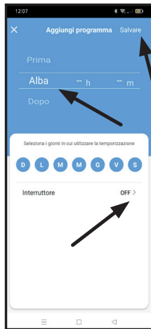
Select sunrise, before or after and how much advance or delay. Then press on the days of the week you will activate the program. Choose ON or OFF. Finally press “Save”.
