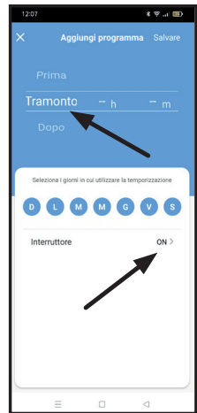
Select sunset, before or after and how much advance or delay. Then press on the days of the week you will activate the program. Choose ON or OFF. Finally press “Save”.
